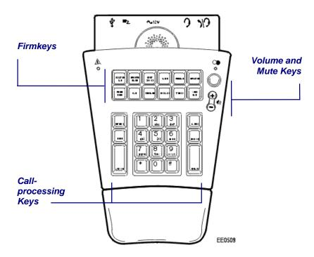
**Volume and Mute Keys** – used to increase (+) or decrease (-) the ringer volume and the volume of the earpiece in the handset or headset. The **Mute** key turns the microphone in the headset or handset on or off.
